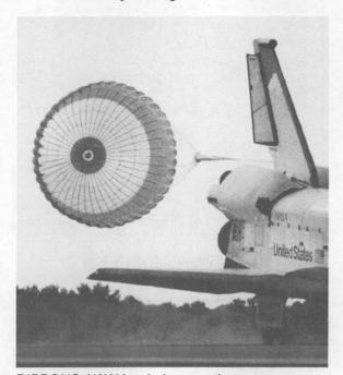
RIBBONS AWAY — Labs parachute experts conducted a series of wind tunnel tests that helped NASA modify parachutes used to slow space shuttle vehicles during landings. Previously, the drag chutes were flying slightly off center.
